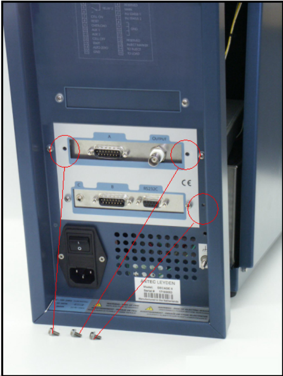
Figure 5. Removal of internal cell cable connector.
