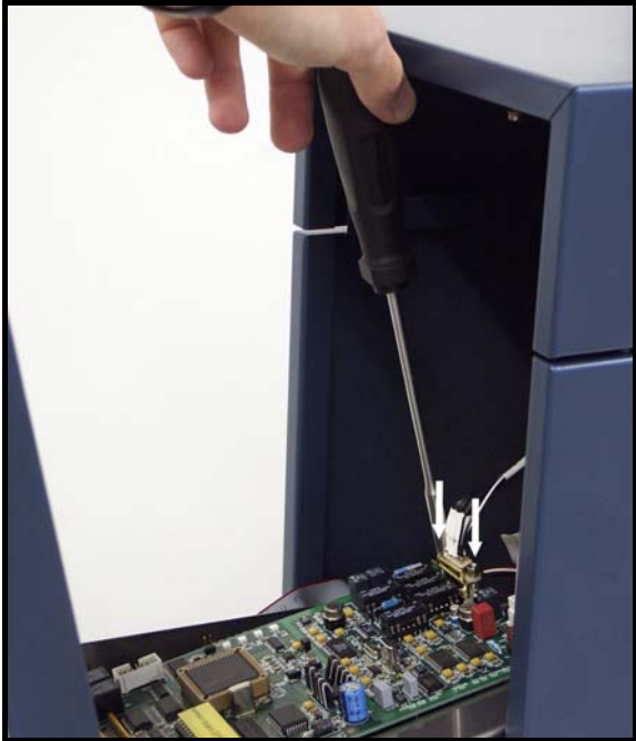
Figure 5. Removal of internal cell cable connector.
